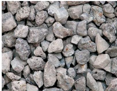
pit run blast furnace slag is extensively used for subbase construction in some areas, especially where weak subgrade conditions exist.
