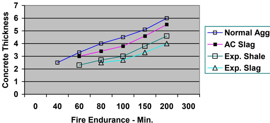
**Fire Resistance of Prestressed Concrete Shapes**
