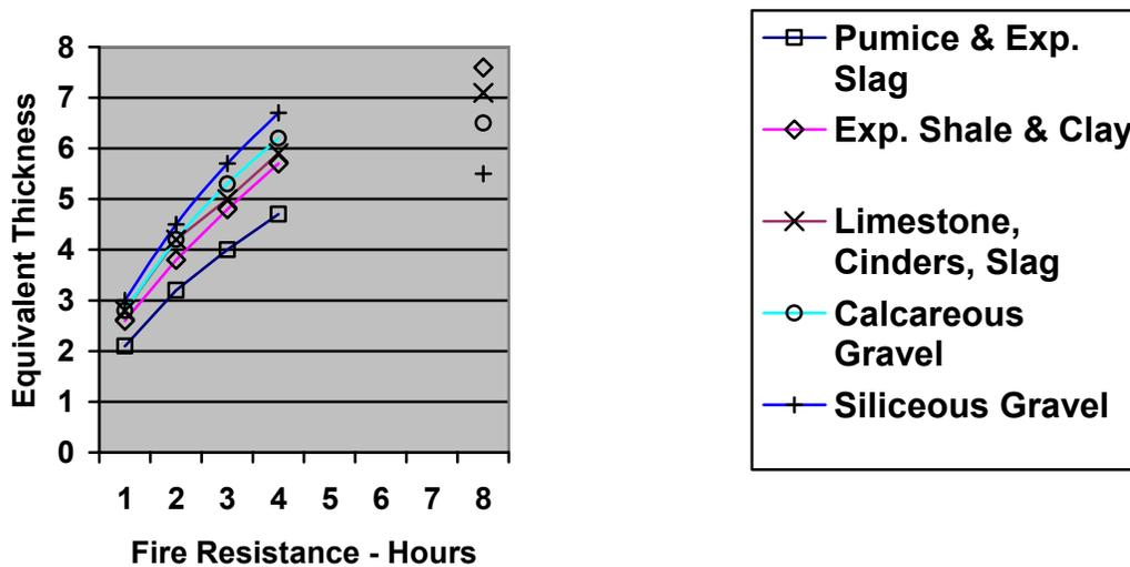
In 1966 full scale ASTM fire tests were performed on various types of masonry units by the Fire Test Sections of the Canadian National Research Council. Based upon these tests a Canadian code shown below has been published.<sup>11</sup> This code shows that slag is far more fire resistant than natural aggregates for all periods of fire resistance ratings.
