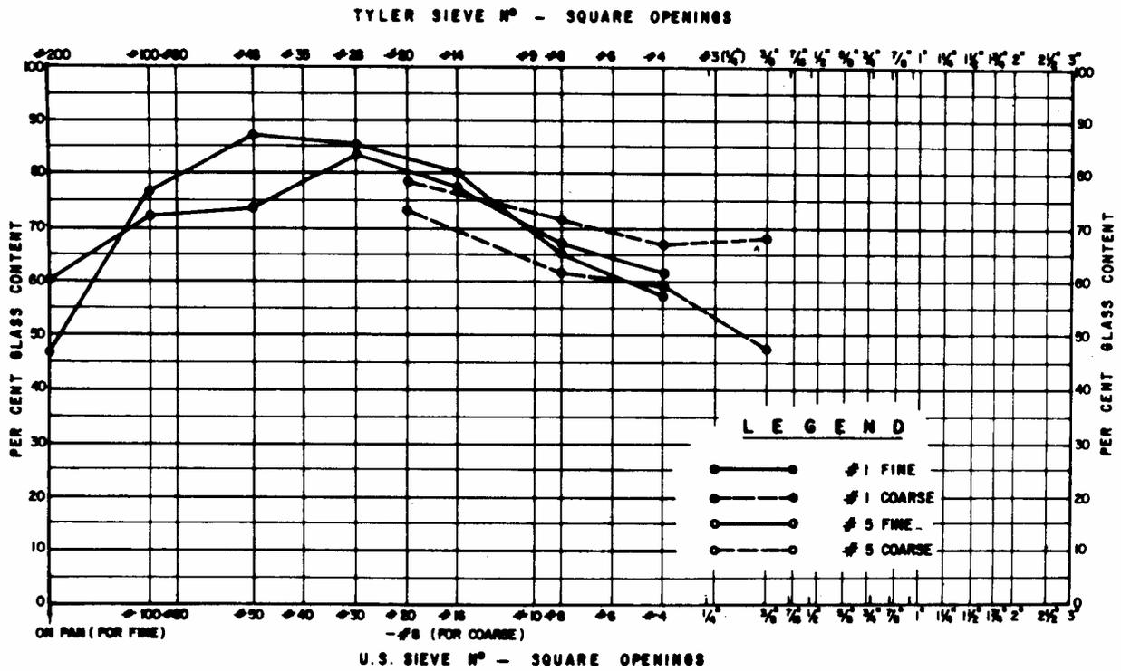
FIG. 4—Glass content for various pellet sizes (McMaster method); refer to Table 1 of ASTM Specifications for Wire-Cloth Sieves for Testing Purposes (E 11-70) for metric equivalents for the alternate sieve designations given.
