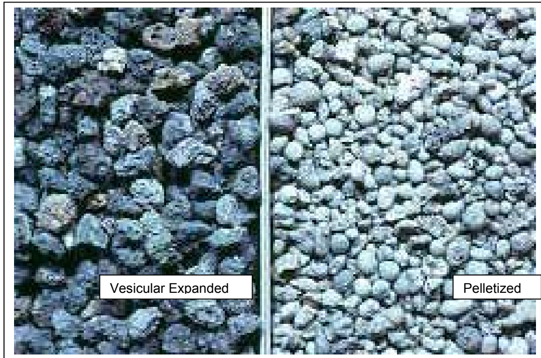
Fig. 3 Comparison of Vesicular Expanded and Pelletized Blast Furnace Slag
