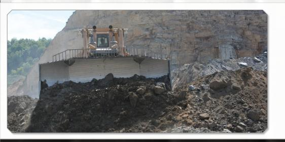
Utilization of a Premium Carbide Overlay Plate to create a very smooth dozer blade liner system.
