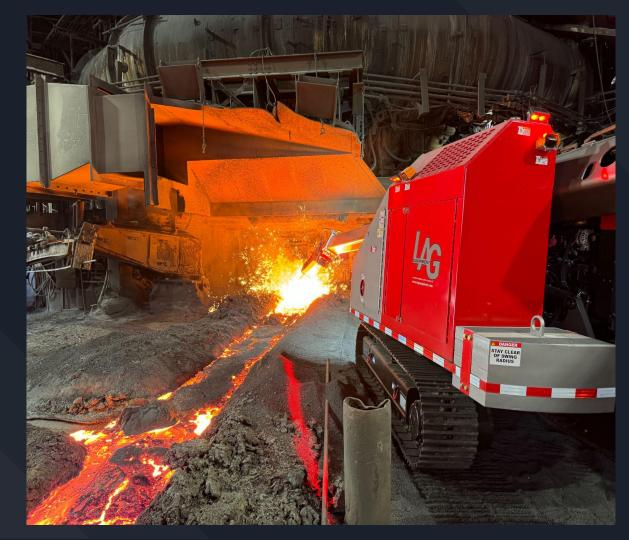
Introducing LAG Equipment's LAG-3400 and LAG-2800 refractory tear-out machines. Taking decades of experience and knowledge, LAG Equipment developed an innovative duo of machines from the ground up, keeping safety front of mind. Using the latest technology, the machines effortlessly tear out refractory or clean out a vessel while allowing the operator to keep a safe distance.
