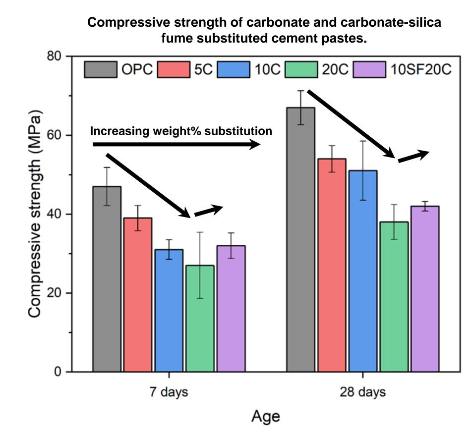
Incorporating a reactive silica phase counteracts the dilution effect of comparatively inert carbonates, allowing for higher substitution levels and improved strength recovery.
